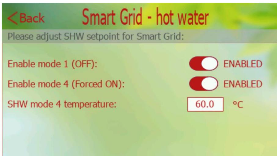
Here it is possible to enable/disable mode 1 (during which domestic hot water heating is disabled), enable/disable mode 4 (during which the highest possible temperature of domestic hot water is required according to the user limit - the use of a bivalent electric heater is possible) and setting the SHW setpoint for mode 4 (higher than the setpoint for normal operation).
