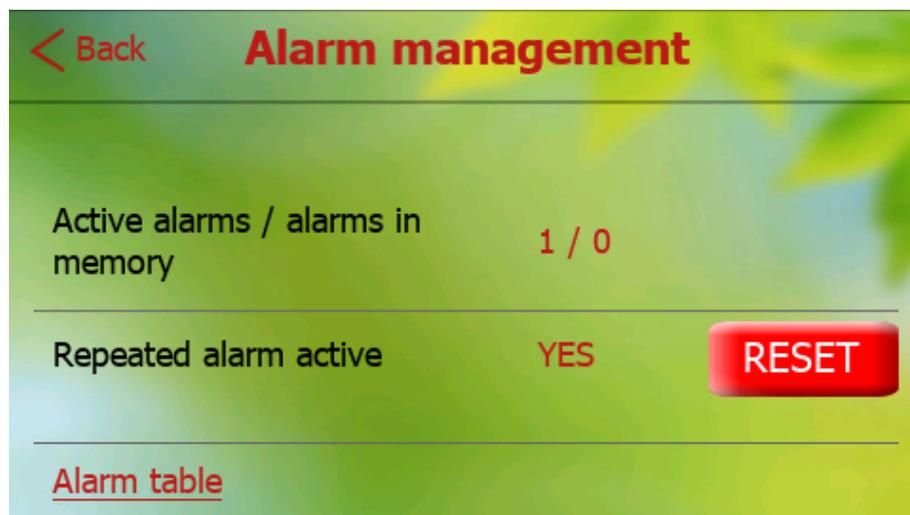
In the picture above we can see **Alarm Management** page. The total number of alarms according to their type is displayed here ([see chapter 11.2 Types of alarms](#)). The second line shows activity of **Repeated alarm** and the button for its **RESET**.
