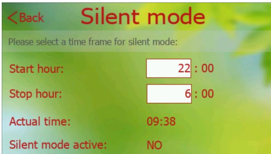
This new function allows night-time sound attenuation (compressor and fan power is reduced) to a minimum level during selected time frame. During this period, an electric heater can be used to replace part of compressor power. This new feature is intended for European countries with the strictest night mode requirements.
