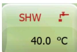
Here it is possible to set the required temperature of sanitary hot water for ECO mode. This value should be lower than the value set in normal mode.
