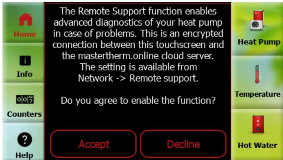
If you agree to the dialog (displayed after updating to version 1114), an authorized specialist will be able to perform advanced diagnostics in case of problems and securely connect to this display and work as if he were standing right in front of it. In case of rejection, it is possible to enable the function in the future or create a secure connection by pressing the appropriate button on the pGDx once.
