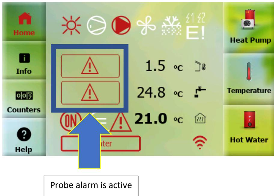
After pressing the alarm button of the sensors, you will be redirected to the page describing this error.
