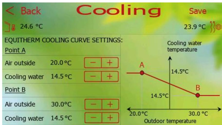
Figure 22 - Cooling curve
