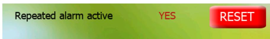
After performing a manual reset, alarm will be transferred to the memory, [see chap. 11.2.3](#). and after the protection time has elapsed (typically 6 minutes) to restore the function of the device. If the function of the device cannot be restored, or occurrence of a repeated alarm occurs more frequently, it is necessary to diagnose cause of the fault and contact installation / service company.
