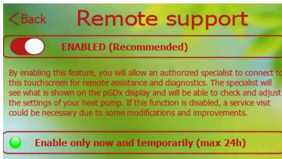
If the feature is **ENABLED**, an authorized technician can connect whenever adjustments, checks or improvements are required.
