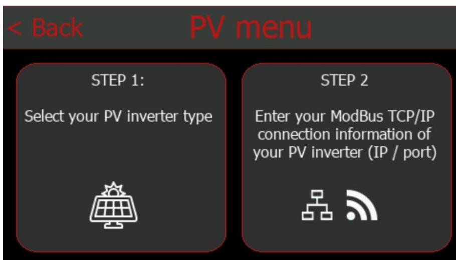
The first step is to select the PV inverter type (only GoodWe and SolarEdge available in this version) or manually enter ModBus TCP/IP addresses:
