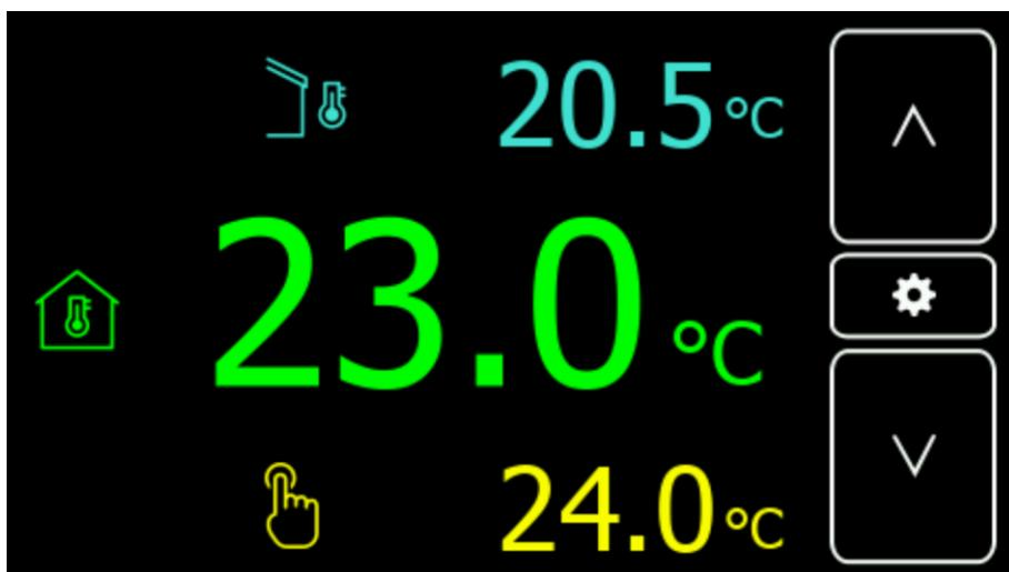
The outdoor temperature, indoor air temperature and desired indoor air temperature are displayed on the screen. Use the up and down arrows to set the value of the desired temperature (in yellow).
