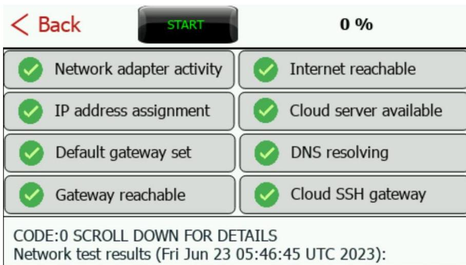
The connection is tested step by step from the local network to the services on our Cloud server. This allows you to find out exactly what the problem is.
