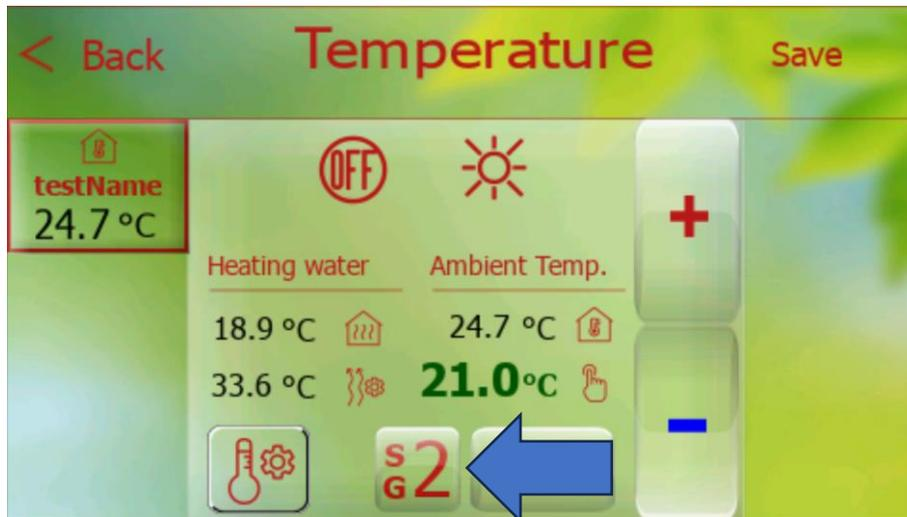
At the same time, after pressing this button, it is possible to quickly switch to the settings of the SmartGrid function for selected heating circuit.
