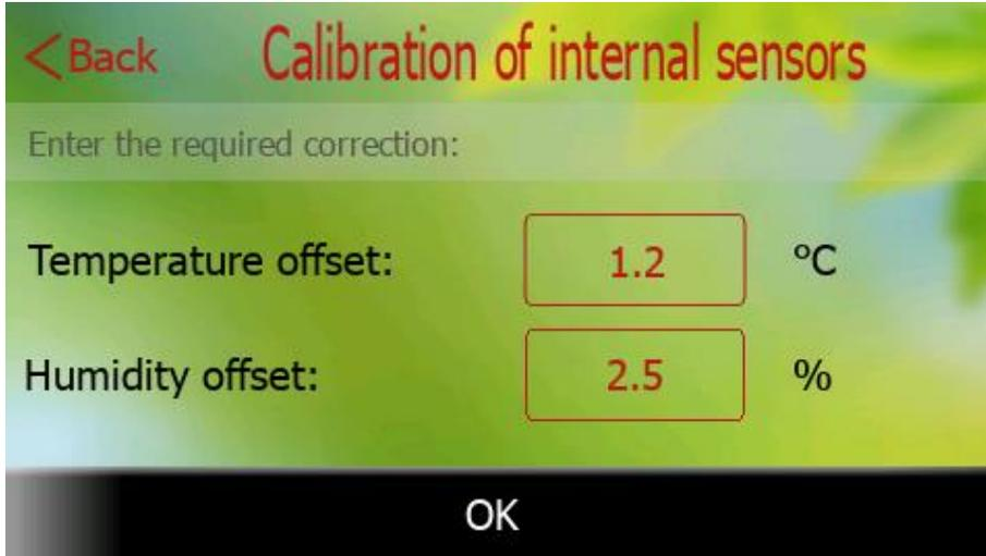
After entering the temperature / humidity correction, press the OK button to confirm and then redirect to the home screen.
