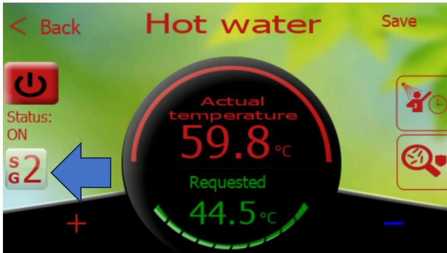
At the same time, after pressing this button, it is possible to quickly switch to the settings of the SmartGrid function for SHW.
