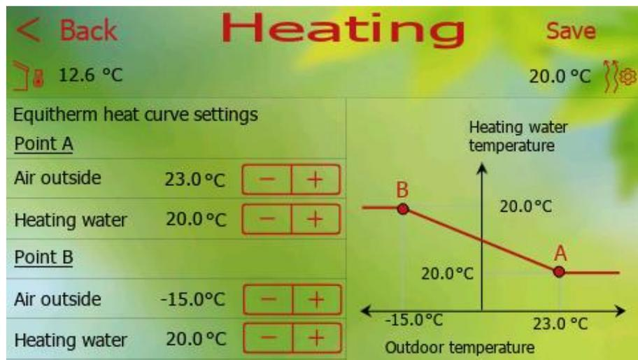
Figure 21 - Heating curve
