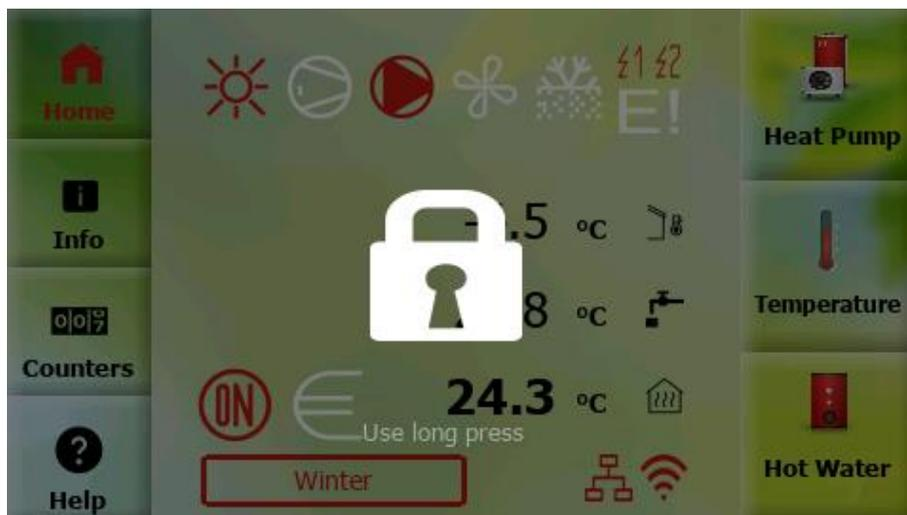
The screen is locked. When you tap the screen, the home screen darkens and the lock icon appears. In case of a long press, the user is redirected to the page for entering the password.
