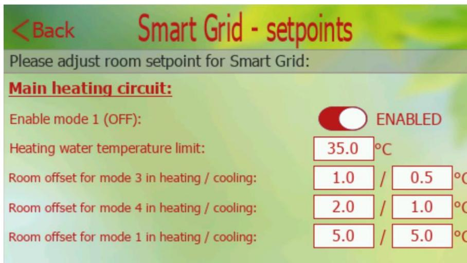
Here it is possible to enable/disable mode 1 (during which heating of the circuit is disabled), adjust the maximum permitted temperature of the heating water of the heating circuit (normally up to 30°C for underfloor heating / higher values can be achieved for radiators), room temperature offset for mode 3 and mode 4 during heating and cooling mode (overheating / undercooling the room by the selected value
