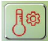
After pressing this button, menu with option to select heating curve or cooling curve (only if cooling function is available) will be expanded
